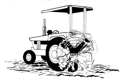
Hitch to the drawbar, or to other specified hitch points. If you hitch to the axle - or anywhere that's too high - the front end will come up FAST and you have only 7/10 of a second to declutch!, or prevent an upset.
