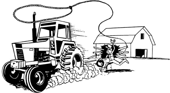
⚠ Engine starting and control operation must be performed from the operators seat only.
