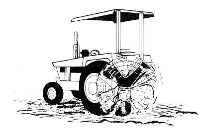
Hitch to the drawbar, or to other specified hitch points. If you hitch to the axle - or anywhere that's too high - the front end will come up FAST and you have only 7/10 of a second to declutch!, or prevent an upset.
