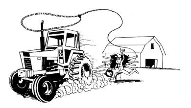
Engine starting and control operation must be performed from the operators seat only.
