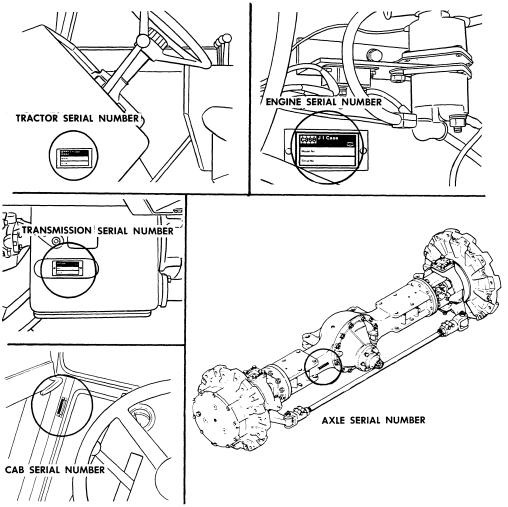
For reference, fill in the Serial Numbers of your tractor in the spaces provided below.
