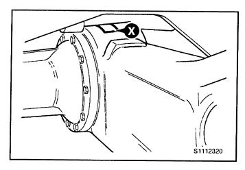
The front axle serial number is stamped on plate Z as shown.
