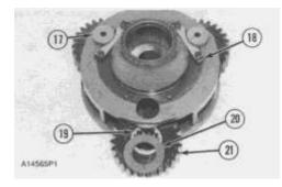
**20.** Bend the locks away from the bolts that hold shafts (17) to the planet carrier. Remove the locks and the bolts. Remove retainers (18) from the shafts.
