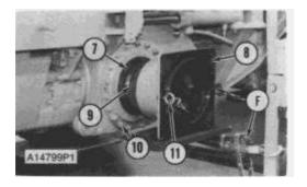
**11.** Install two 5/8" - 11 NC forged eyebolts (11) and nuts in the housing as shown. Put a fork lift truck in position under the housing. Install tooling (F) on the lift truck and the eyebolts.
