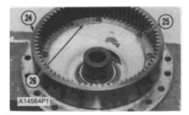
**23.** Bend the locks away from bolts (25). Remove bolts (25). Remove plates (26) that hold ring (24) to the housing.
