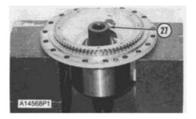
25. Remove shaft (27) from the housing. Weight is 18 kg (40 lb.).
