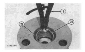
**22.** Remove ring (23) from the planet carrier with tooling (I). Remove washer (22) from the planet carrier.
