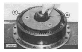
**19.** Remove pinion (16) from planet carrier (15). Fasten a hoist to planet carrier (15) and remove it. Weight is 41 kg (90 lb.).
