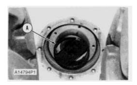
${f 1.}$  Remove the nut that holds the sprockets on the shaft with tooling (A). Install tooling (B) on the shaft.
