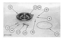
19. Remove twenty springs (23) and twenty springs (24) from parking brake housing (12).
