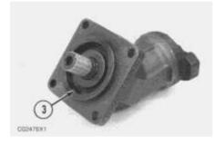
**4.** Tap the cover with a plastic hammer to release some of the pressure against retaining ring (3). Use tool (A), and remove retaining ring (3).
