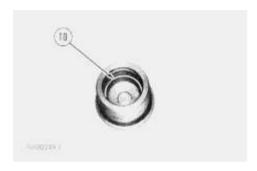
7. Remove bearing cup (10) from the pinion cap.
