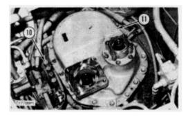
4. Remove four bolts (10) from each side of swing drive (11).
