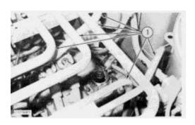
**1.** Remove six hydraulic tube assemblies (1).
