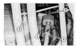
**2.** Remove two bolts and block (2) that fasten the parking brake cable to the housing. Disconnect hose assembly (4) and tube assembly (3) from bracket (5).
