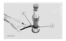
**5.** Remove snap ring (6) from pinion cap with tool (A). Remove the cap.
