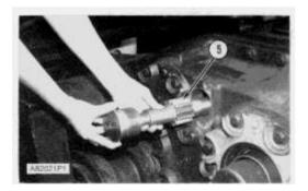
**4.** Remove disconnect pinion (5) and the O-ring seal from the pinion.
