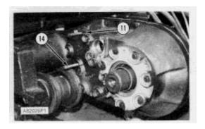
**9.** Install two 5/8" - 11 NC forcing screws (14) in cage (11) and remove the cover, shims and the O -ring seal.
