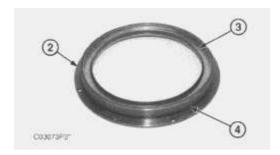
2. Remove O-ring seal (4) and crankshaft seal (3) from adapter (2).
