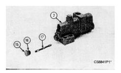
**8.** Remove O-ring seal (16) from plug (15). Remove spool (17) from pressure valve (2).
