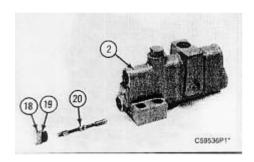
9. Remove plug (18), O-ring seal (19) and spool (20) from pressure valve (2).
