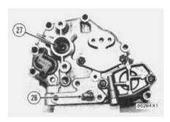
12. Remove seal (27) and adjustment screw (28) for the high idle.
