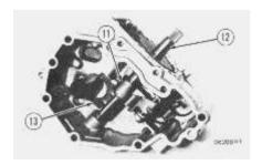
**5.** Remove shaft assembly (12), lever (11) and lever (13) from the housing.
