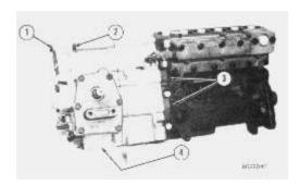
1. Remove bolt (1), six bolts (2), two top bolts (3), housing (4) and the gasket.
