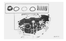
**2.** Remove governor spring (5), the two wave washers, one flat washer and seat from the guide in the housing.
