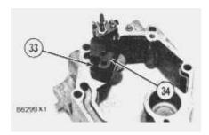
**16.** Remove bolts (33) and block (34) for the full load stop from the housing.
