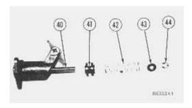
**20.** Remove lockring (44), seat (43), spring (broken link spring) (42) and sleeve (41) from valve (40). Remove the other lockring (44) from the groove in the center of valve (40).
