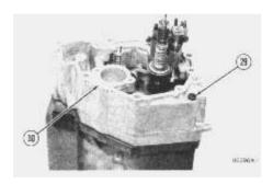
13. Remove two bolts (29), housing (30) and the gasket from the fuel injection pump housing.
