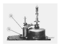
19. Remove bolts (39) and governor servo (38) from the fuel injection pump.
