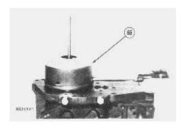
**31.** Use a screwdriver to remove shield (66) as shown.
