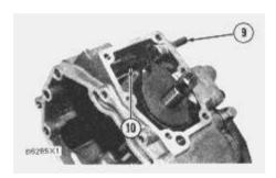
**4.** Remove low idle adjustment screw (9) and spring (10) from the housing.
