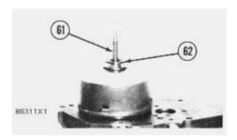
29. Remove spring (overfueling spring) (61) and riser (62) from the governor shaft.
