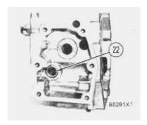
9. Remove check valve (22) if a replacement is necessary.
