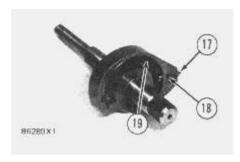
7. Remove pin (18), pin (17) and spring (19) from the shaft assembly.
