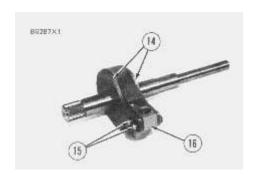
**6.** Remove two snap rings from pins (15) and remove pins (15). Remove plates (14) and stop (16) from the shaft assembly.
