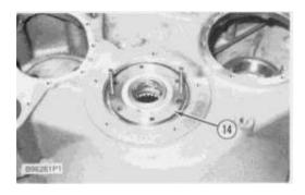
**13.** Remove the bolts that hold manifold (14) to the case assembly. Install two 3/8"-16 NC forcing screws in the manifold. Tighten the forcing screws evenly, and remove the manifold from the case assembly.
