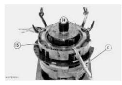
14. Use tools (C) to hold the piston in number six clutch housing (15).
