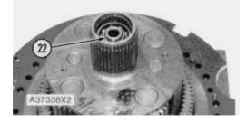
**19.** Remove ring (22) from the intermediate shaft. The ring holds the bearing on the intermediate shaft.
