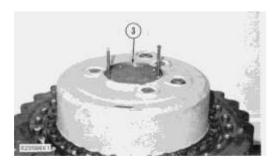
**4.** Remove the bolts that hold cover (3) in place, and use two 3/8"-16 NC forcing screws to remove the cover.
