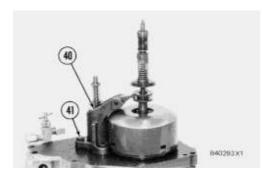
**21.** Remove bolts (41) and governor servo (40) from the fuel injection pump.
