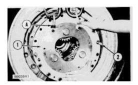
**3.** Fasten tooling (A) and a hoist to the planet carrier. Put final drive planet carrier (1) in position in the wheel assembly. Install the bolts that hold it. Remove guide bolts (2). Install the remainder of the bolts. Tighten the bolts to a torque of  $150 \pm 20$  lb.ft. ( $205 \pm 27$  N·m).
