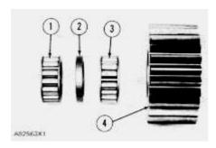
1. Install bearings (1) and (3) and spacers (2) in gears (4).
