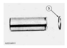
**2.** Install retainer rings (5) on the shaft.
