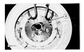
**2.** Fasten tooling (A) and a hoist to the final drive planet carrier as shown. Remove the remainder of the bolts that hold the final drive planet carrier to the wheel assembly.
