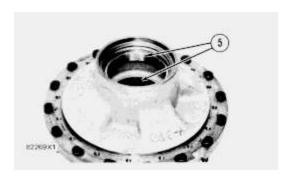
**4.** Remove bearing cups (5) from the wheel assembly.
