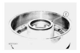
**2.** Remove Duo-Cone seal (2) from the wheel assembly.
