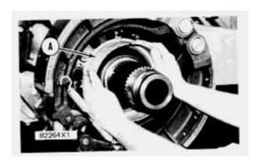
2. Make sure the rubber torus seals are clean and dry. Make sure all metal surfaces that make contact with the rubber torus seals are clean and dry. Use tool (A) to install the Duo-Cone seal in the retainer. Put a small amount of clean SAE 30 oil on the surfaces of the metal seals that make contact with each other.
