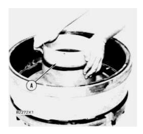
**6.** Make sure rubber torus seals are clean and dry. Make sure all metal surfaces that make contact with the rubber torus seals are clean and dry. Use tool (A) to install the Duo-Cone seal in the wheel assembly. Put a small amount of clean SAE 30 oil on the surfaces of the metal seals that make contact with each other.
