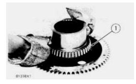
**1.** Heat the bearing cone to a maximum temperature of  $275^{\circ}$  (135°C). Install bearing cone (1) on the hub.
