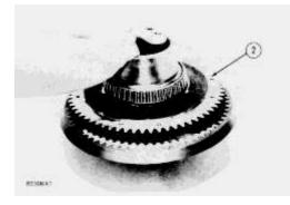
2. Put hub assembly (2) in position in the ring gear.
