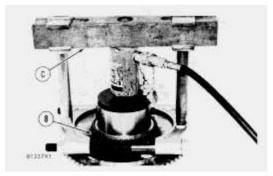
**6.** Use tooling (C) to remove bearing cone (8) from the hub.
