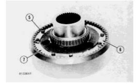
**5.** Remove bolts (5). Remove locks (6) and plates and remove hub assembly (7) from the ring gear.
