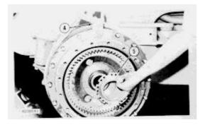
5. Install nut (5) on the spindle. Remove tool (A) and the hoist from the wheel assembly.
