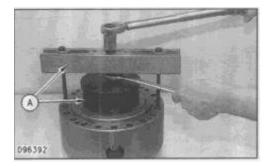
**b.** Tighten the center bolt of Tooling (A) to a torque of **27** N·m (**20** lb ft) to apply **900** kg (**2000** lb) of preload on the disc packs.
