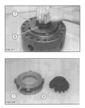
5. Remove actuator housing (7) and gear (8) from the case housing, as shown.
