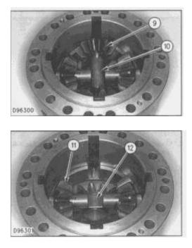
6. Remove pinion shaft (10) and two pinion gears (9).
