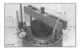
e. Carefully remove Tooling (B) from the case cover.
