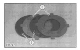
**5.** Remove the disc pack from the case housing. The disc pack consists of two friction discs (5) and two plates (6).
