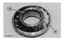
**38.** Remove retaining ring (50) from stator (48).
