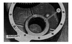
**12.** Use tooling (C) to remove bearing cup (15) from the cover assembly.
