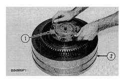
3. Put cover (1) in position on rotating housing (2). Install the bolts and washers that hold cover (1) in place. Tighten the bolts to a torque of  $30 \pm 5 \text{ N} \cdot \text{m}$  (22 \pm 4 lb ft).
