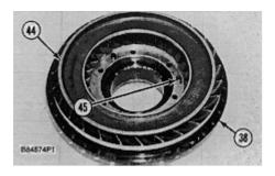
**33.** Remove impeller (44) from drive flange (38). If necessary, remove dowels (45) from the drive flange.
