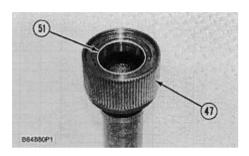
**39.** Remove sleeve bearing (51) from carrier assembly (47).
