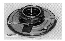
31. Remove bolts (43) and washers (42) that hold the hub and impeller to the drive flange.
