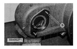
**21.** If necessary, remove studs (28) from the cover assembly.
