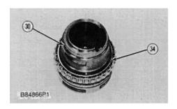
**25.** Remove retaining ring (34) from bearing carrier (30).
