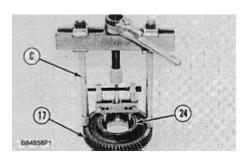
17. Use tooling (C) to remove bearing cup (24) from transfer gear (17).
