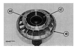
**36.** Remove retaining ring (48) that holds stator (49) to carrier assembly (47).
