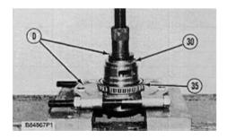
**26.** Use tooling (D) and a press to remove inner bearing (35) from bearing carrier (30).
