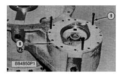
**8.** Use three 3/8" - 16 NC forcing screws (9) to remove pump adapter (8) from the cover assembly.
