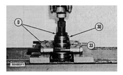
24. Use tooling (D) and a press to remove ring carrier (33) from bearing carrier (30).
