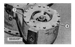
7. Remove bolts (7) and the washers that hold pump adapter (8) to the cover assembly.
