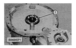
1. Remove bolts (1) and the washers that hold the torque converter to the cover assembly.
