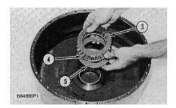
**4.** Put thrust bearing race (5), thrust bearing (4), and thrust bearing race (3) in position on the cover.
