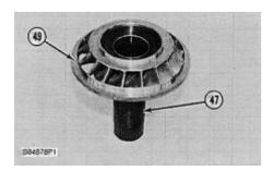
**37.** Heat stator (49) and carrier assembly (47) as a unit to a **minimum temperature of 121°C** (250°F) for one hour to expand the stator. Remove stator (49) from carrier assembly (47).
