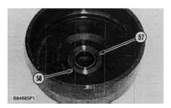
44. Remove two thrust bearing races (57) and thrust bearing (58) from the cover assembly.
