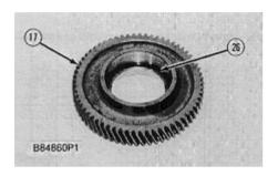
**19.** Remove retaining ring (26) from transfer gear (17).
