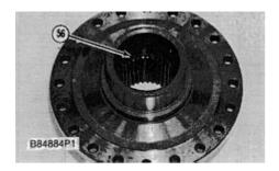
**43.** Remove retaining ring (56) from the hub.
