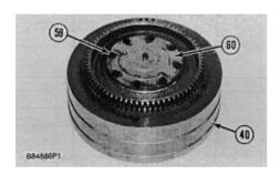
**45.** Remove bolts (59) and the washers. Remove cover (60) from rotating housing (40).
