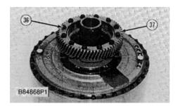
27. Remove bolts (36) and the washers and drive gear (37) from the drive flange.
