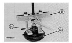
11. Use tooling (B), and remove bearing cones (14) from each side of pump gear (13).
