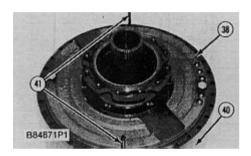
**30.** Use two 5/16" - 18 NC forcing screws (41) to remove drive flange (38) from rotating housing (40). The weight of the drive flange is **23 kg (51 lb).**
