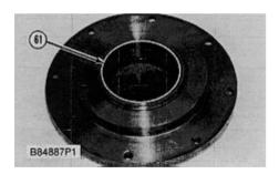
**46.** Remove sleeve bearing (61) from the cover.
