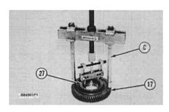
**20.** Use tooling (C), and remove bearing cup (27) from transfer gear (17).
