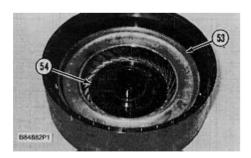
**41.** Remove turbine (53) and hub (54) as a unit from the rotating housing.
