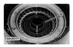
**40.** Remove thrust race (52) and the thrust bearing from the hub.
