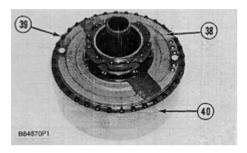
29. Remove bolts (39) that hold drive flange (38) to rotating housing (40).
