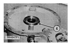
**4.** Remove O-ring seal (4) from the cover assembly.
