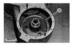
**10.** Remove pump gear (13) from the cover assembly.
