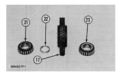
16. Remove bearing cone (21), spacer (22) and bearing cone (23) from transfer gear (17).
