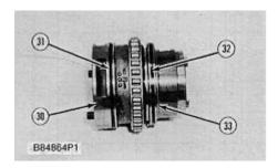
23. Remove O-ring seal (31) from bearing carrier (30) and seal ring (32) from ring carrier (33).
