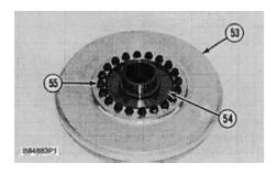
**42.** Remove bolts (55) and the washers. Remove turbine (53) from the hub (54).
