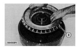
7. Put turbine (8) and the hub as a unit in position in the housing. Check the clearance between the hub and sleeve bearing in the cover. The clearance must be  $0.150 \pm 0.051$  mm (.0059  $\pm$  .0020 in).
