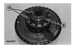
22. Remove retaining rings (29) and bearing carrier (30) from the carrier assembly.
