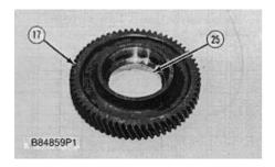
**18.** Remove spacer (25) from transfer gear (17).
