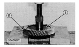
**28.** Use tool (E) and a press to remove the outer bearing race from drive gear (37).
