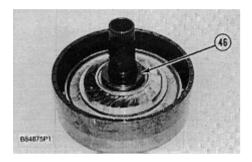
**34.** Remove two thrust bearing races (46) and the thrust bearing from the carrier assembly.
