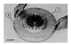
6. Put turbine (8) in position on hub (7) as shown. Install the bolts that hold the turbine in place. Tighten the bolts to a torque of  $55 \pm 10 \text{ N} \cdot \text{m}$  (40 ± 7 lb ft).
