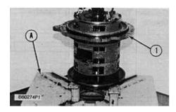
7. Put planetary group (1) in position on tool (A) as shown. Fasten the planetary group to tool (A) with suitable size bolts, washers and nuts.
