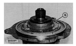
**17.** Remove ring gear (16) from the manifold assembly.
