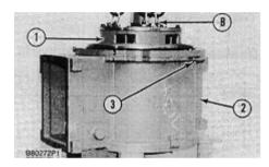
**3.** Fasten tool (B) and a hoist to planetary group (1). Remove bolts (3) that hold transmission case (2) to planetary group (1).
