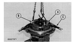
**11.** Use tool (C) to hold the clutch piston in No. 6 clutch housing (8).
