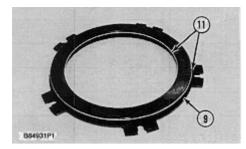
14. Remove seal rings (11) from clutch piston (9).
