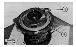
8. Remove two O-ring seals (5) and O-ring seal (6) from the manifold assembly.
