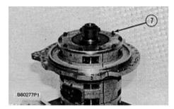
**9.** Put an alignment mark across the clutch housing assemblies of the planetary group for assembly purposes.
