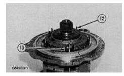
15. Remove five dowels (12) and springs (13) from the manifold assembly.
