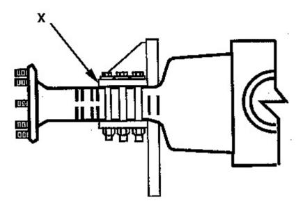
**8.** On the opposite side of the machine, measure the gap (X) between the axle and the frame.
