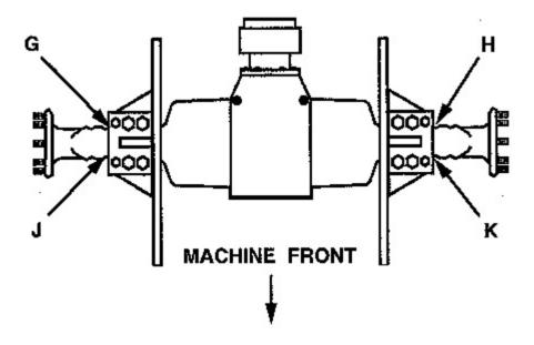
9. Measure the gap at locations (G) and (J). If the gap is less than 1.5 mm (.06 in), repeat Steps 6 and 7 on the remaining side. If the gap at location (G) or (J) is greater than 1.5 mm (.06 in), install one 1G-8271 Shim. If the gap at location (G) or (J) is greater than 2.5 mm (.10 in), install one 1G-8271 Shimon each side of the frame. Use one shim in the gap and one shim diagonally across the gap between the frame and axle.
