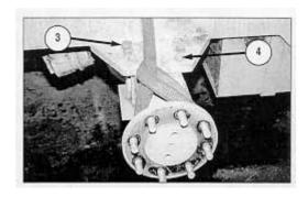
**3.** Remove four bolts (3) and two bolts (4) from each end of the axle.
