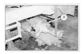
**4.** Use the lifting device to lower axle (2) to a dolly or similar device. The weight of the axle is **385 kg (850 lb).**
