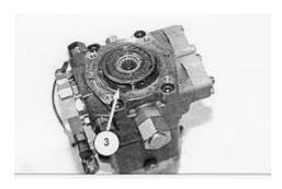
**2.** Remove O-ring seal (3) from the charge pump. Check the O-ring seal for wear or damage, and replace if necessary.
