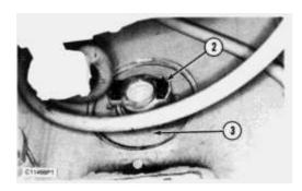
**2.** Remove drive shaft yoke (2). Use forcing bolts and remove retainer (3) and the O-ring seal from the transmission and bevel gear case.
