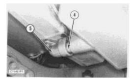
**4.** Remove elbow (5) from the bottom of the flywheel housing. Remove the O-ring seal from elbow (5).
