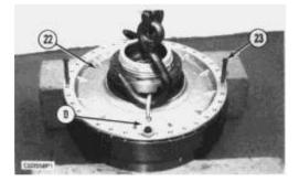
**19.** Remove the remaining thirty-four bolts (15) and washers. Install two 3/8 "-16 NC forcing screws (23) into impeller wheel (22).
