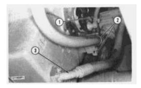
**2.** Loosen the flange bolts on hose (3) and drain the oil from the torque divider. Disconnect hose (3) from the torque divider when the oil has drained. Remove the O-ring seal from hose (3).
