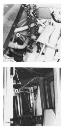
6. The weight of the torque divider is 145 kg (320 lb). Install tooling (A) onto the torque divider.
