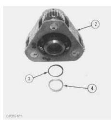
**3.** Remove retainer (4) and retaining ring (3) from the planetary carrier.
