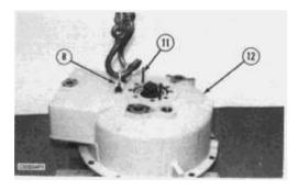
**11.** The weight of cover (12) is **68 kg (150 lb)**. Install tooling (B), and attach a hoist. Install two 3/8 "-16 NC forcing screws (11) in the cover. Tighten the forcing screws evenly, and remove cover (12).
