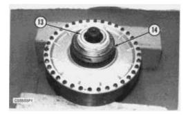
12. Remove O-ring seal (14) and lip-type seal (13).
