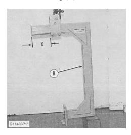
**4.** Adjust the top bracket on Tooling (B) so that distance (X) is **213 mm (8.4 in)**. The lower mounting bracket must be installed with the spacers outward as shown.
