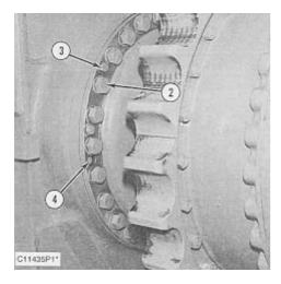
**5.** Remove two of the bolts from the sprocket segment. Fasten a hoist and install Tooling (B) onto the final drive.
