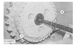
1. Turn the final drive until drain plug (1) is on the bottom as shown. Remove drain plug (1) and drain approximately 13.2 liters (3.4 U.S. gal) of oil from the final drive.
