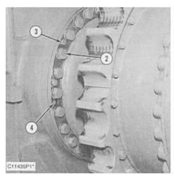
**5.** Remove two of the bolts from the sprocket segment. Fasten a hoist and install Tooling (B) onto the final drive.
