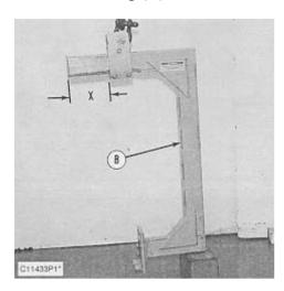
**4.** Adjust the top bracket on Tooling (B) so that distance (X) is **213 mm (8.4 in)**. The lower mounting bracket must be installed with the spacers outward as shown.
