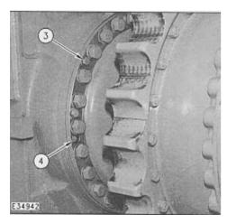
**3.** Fasten a hoist and install Tooling (B) on the final drive. Adjust Tooling (B) if necessary to put the final drive in a level position.
