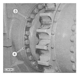
**5.** Remove two of the bolts from the sprocket segments. Fasten a hoist and install Tooling (B) on the final drive.
