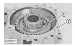
**8.** Remove transfer gear (11) from transfer gear case (3).
