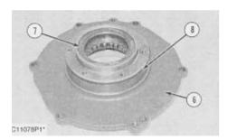
**6.** Remove lip-type seal (7) and O-ring seal (8) from cage (6).
