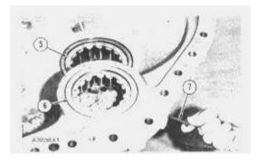
7. Remove the dowel for race and roller assembly (6) with a 10-32 screw (7). Remove the dowel for race and roller assembly (5) with a 1/4"-20 NC bolt.
