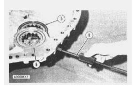
**6.** Remove the plugs for the dowels that hold race and roller assemblies (5) and (6) in place with tooling (B).
