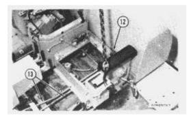
**8.** Fasten a hoist to seat frame assembly (12). Remove the seat frame assembly. Weight of the seat frame assembly is 115 lb. (52 kg).
