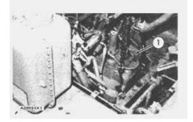
**1.** Install four 5/8" - 11 NC forged eyebolts or tooling (A) on the transmission and transfer gears. Fasten a hoist. Put transmission and transfer gears (1) in position on the bevel gear case. Install the washers and nuts that hold the transmission and transfer gears to the bevel gear case. Remove the hoist.
