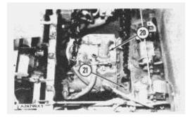
**13.** Install four 5/8" - 11 NC forged eyebolts or tooling (A) on the transmission and transfer gears. Fasten a hoist. Remove nuts (21) that hold the transmission and transfer gears to the bevel gear case. Remove the transmission and transfer gears. The weight is 1150 lb. (522 kg).
