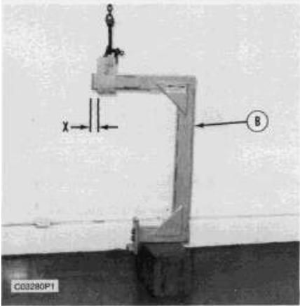
5. Adjust the lifting shackle on tooling (B) so distance (X) is **38 mm (1.5 in)**. The lower mounting bracket should be installed so the spacers are out as shown.
