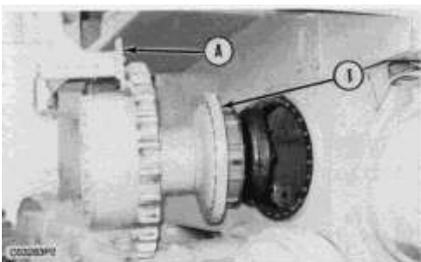
2. Fasten a hoist, and install tooling (A) on the final drive. Make an adjustment to tooling (A), if needed, to level the final drive and steering clutch and brake.
