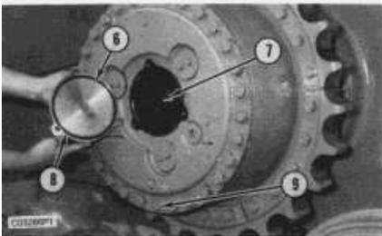
9. Install retainer (7) into the sun gear.
