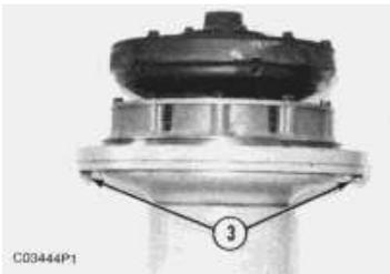
2. Remove two bolts (3) from the steering clutch and brake.
