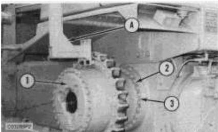
3. Fasten a hoist, and install tooling (A) on final drive (1). Make an adjustment to tooling (A) if necessary to put the final drive in a level position. Put final drive (1) in position on the machine.
