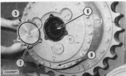
8. Install retainer (6) into the sun gear.
