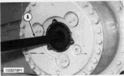
3. Remove the retainer from the sun gear.
