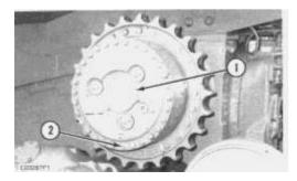
1. Turn the final drive until drain plug (2) is on the bottom as shown. Remove drain plug (2) and drain approximately 11.4 liter (3 U.S. gal.) of oil from the final drive.
