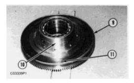
7. Remove ring (9) and spring (11) from retainer (10).
