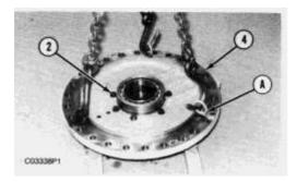
**6.** Turn the brake group over, and install tooling (A). The weight of brake housing (4) is **73 kg (161 lb)**. Remove seven bolts (2). Use a soft hammer, and remove brake housing (4) from the retainer.
