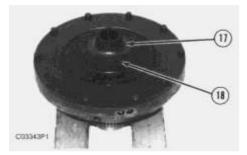
**13.** The weight of the steering clutch group is **159 kg (350 lb)**. Remove four bolts (18) and hub (17).
