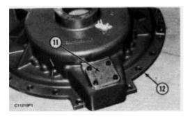
**12.** The weight of transmission cover (12) is **100 kg (220 lb)**. Install tooling (C) to the transmission cover, and fasten a hoist. Remove the transmission cover from tooling (A).
