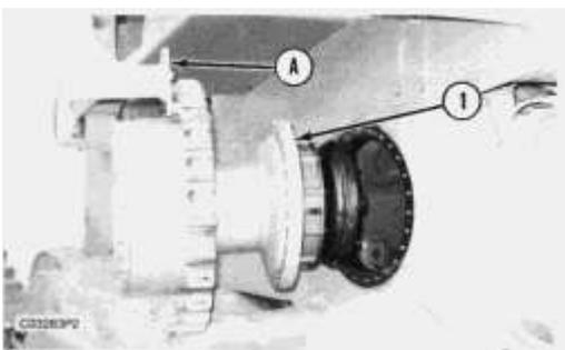
2. Fasten a hoist, and install tooling (A) on the final drive. Make an adjustment to tooling (A), if needed, to level the final drive and steering clutch and brake.
