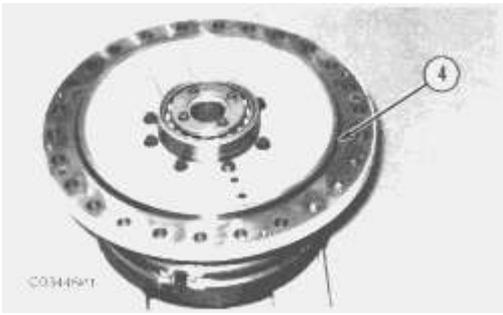
5. Turn the steering clutch and brake over. Remove O-ring seal (4).
