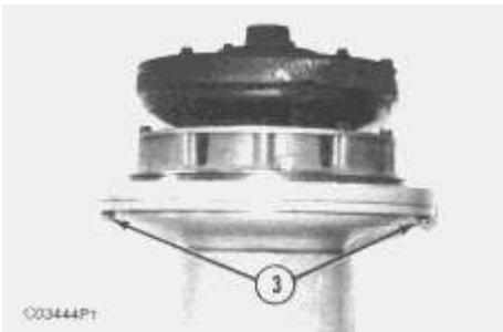
2. Remove two bolts (3) from the steering clutch and brake.
