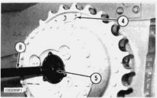
6. Put **SAE 30** oil on the threads of two segment bolts (4). Install the bolts and nuts with the head of the bolts and washers against the final drive. Tighten the nuts to a torque of **300 ± 50 N·m (221 ± 37 lb ft)**. Tighten the nuts 1/3 turn more. Final torque must be a minimum of **570 N·m (420 lb ft)**.
