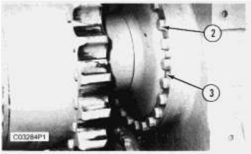
4. Install two bolts (3) that hold the steering clutch and brake to the frame.
