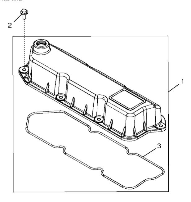
John Deere > Turf And Utility >TRACTOR >5065E - TRACTOR >5065E Tractor (IT4)(9X3 TSS Transmission W/ Cab)(12X12 PR Transmission W/ Cab and OOS) (North America Edition) >20 ENGINE 3029TPY22 >ST614040 - 1125 ROCKER ARM COVER
