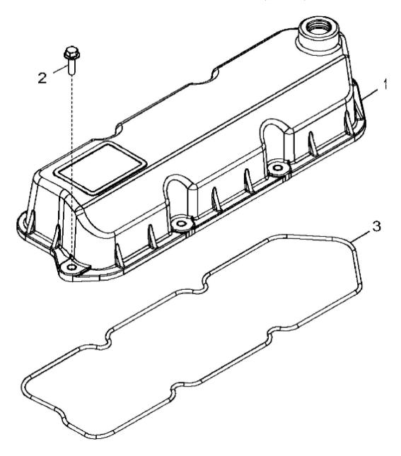
John Deere > Turf And Utility >TRACTOR >5075E - TRACTOR >5075E Tractor (IT4)(9X3 TSS Transmission W/ Cab)(12X12 PR Transmission W/ Cab and OOS) (For Europe, Australia, New Zealand, JDLA, Sub-Saharan Africa and Mexico) >20 ENGINE 3029HPY40-DZ100016 >ST757957 - 11AA ROCKER ARM COVER ( - XXXXXXX)
