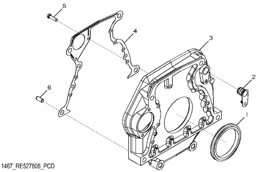
John Deere > Turf And Utility >TRACTOR >5065E - TRACTOR >5065E Tractor (9X3 TSS Transmission W/ OOS)(Asia Edition) >20 ENGINE 3029TPY67-DZ10406-DZ10406 >ST614045 - 1467 FLYWHEEL HOUSING
