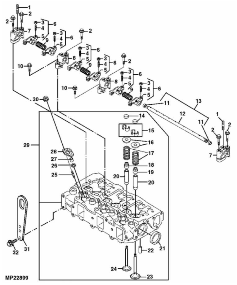
John Deere > Turf And Utility >TRACTOR, COMPACT UTILITY >4200 - TRACTOR, COMPACT UTILITY >4200 Compact Utility Tractors >20 ENGINE >ST638677 - CYLINDER HEAD, VALVES AND ROCKER ARMS
