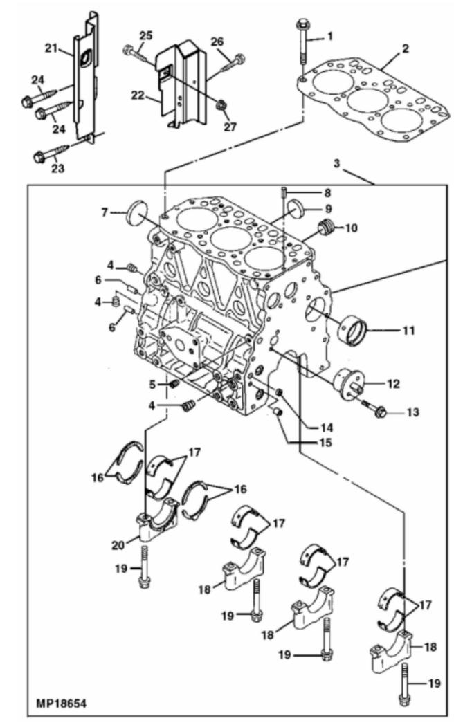
John Deere > Turf And Utility >TRACTOR, COMPACT UTILITY >4200 - TRACTOR, COMPACT UTILITY >4200 Compact Utility Tractors >20 ENGINE >ST638676 - CYLINDER BLOCK AND MAIN BEARINGS
