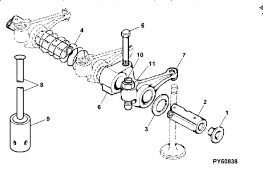
John Deere > Turf And Utility > TRACTOR > 5203S - TRACTOR > 5310 (S.N. PY5310S005119- ) and 5203S (S.N. PY5203S000001 -) Tractors (India Edition) > 20 ENGINE > ST665160 - ROCKER ARM SHAFT
