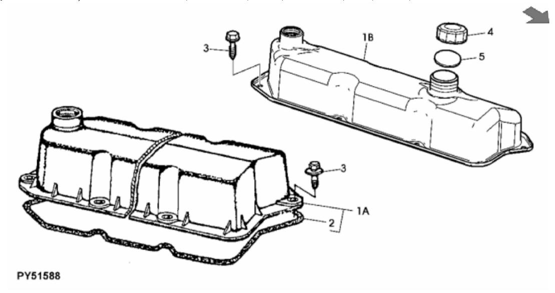
John Deere > Turf And Utility > TRACTOR > 5203S - TRACTOR > 5310 (S.N. PY5310S005119- ) and 5203S (S.N. PY5203S000001 -) Tractors (India Edition) > 20 ENGINE > ST665158 - VALVE COVER
