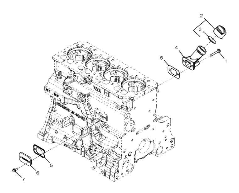
John Deere > Turf And Utility >TRACTOR >5090G - TRACTOR >5090G Tractor (Engine 4045HAT81)(Europe Edition) >20 ENGINE 4045HAT81-DD21693 >ST52635 - 1231 OIL FILLER NECK
