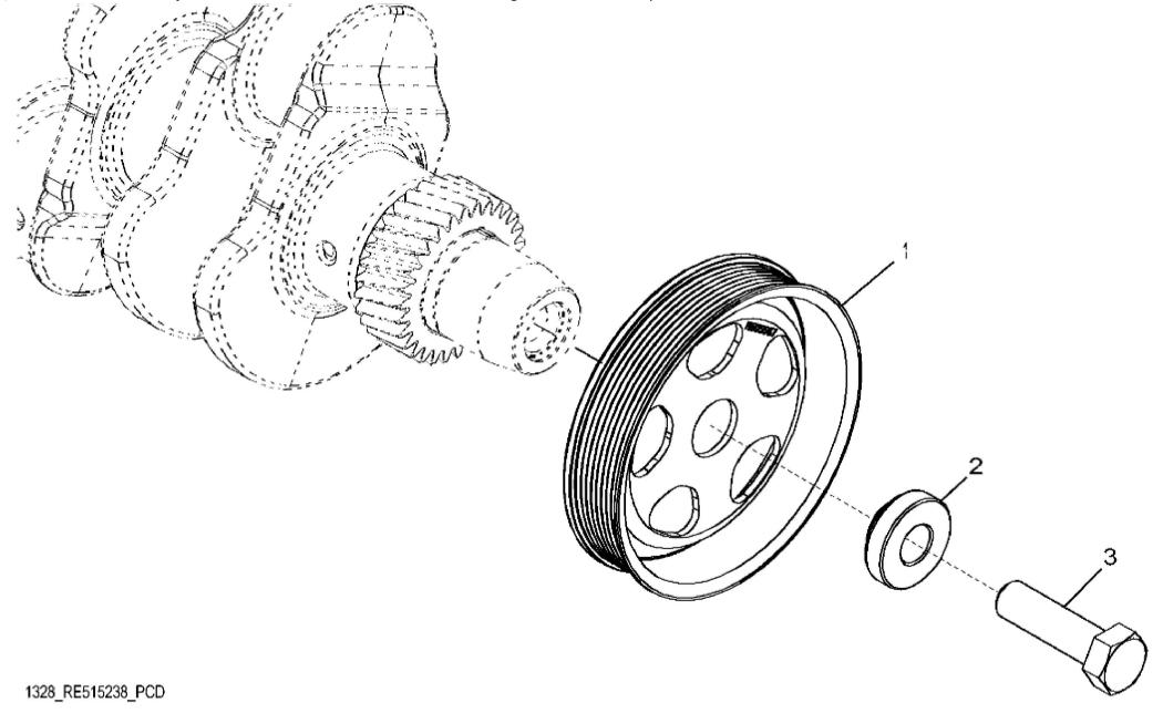
John Deere > Turf And Utility >TRACTOR >5080GV - TRACTOR >5080GV Tractor (Engine 4045HAT80)(Europe Edition) >20 ENGINE 4045HAT80-DD21692 >ST628039 - 1328 CRANKSHAFT PULLEY
